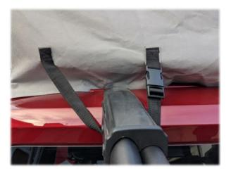
Your California roof cover will fit securely to your Volkswagen California providing increased insulation and protection to the roof bellows. To remove the cover simply follow the instructions in reverse, remembering to undo all clips prior to lowering roof, then remove the rear corners first for ease of removal.
